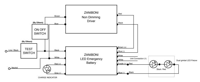
(1) DO NOT CONNECT UNTIL INSTALLATION IS COMPLETE AND AC POWER IS SUPPLIED
